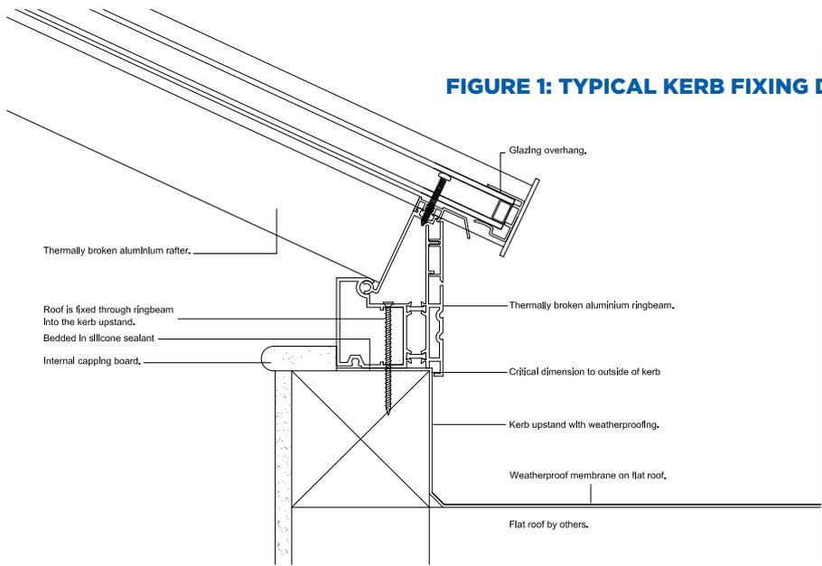
**FIGURE 1: TYPICAL KERB FIXING DETAIL**
